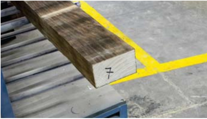
The outer surface of acetylated lumber is caramelised to a darker colour to a depth of 3-10 mm.
